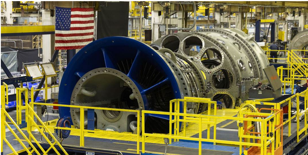
A turbine being assembled at GE Vernova's Greenville, S.C., manufacturing plant. GE VERNOVA
